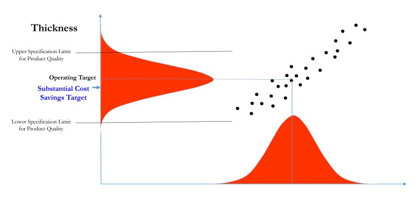
Sawing Deviation / Feed Speed
