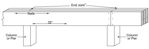
\*Beam continuity is maintained by staggering end joints of adjacent plies.
