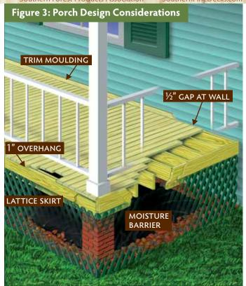
Attention to proper porch design is as important to the longevity of the structure as are the details of porch flooring specification and installation. Inadequate air circulation beneath the porch and trapped moisture between framing components will greatly reduce the serviceability and long-term appearance of the porch. The following recommendations are key elements to the proper design and construction of a fully-covered porch:
