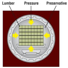
Cross-section of pressure cylinder
